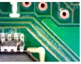
Figure 4: Board cleaned with brush attachment (no separate aerosol was used). No pre-rinse or final rinse utilized. White residue shown around QFN B and QFP, respectively.
