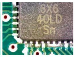
Figure 2: Board cleaned with handheld brush. The components were wetted, and then the brush was wetted and used to scrub the contaminated area. The board in the first picture did not undergo a final rinse. The board in the second picture did (Note: all flux was not removed).
